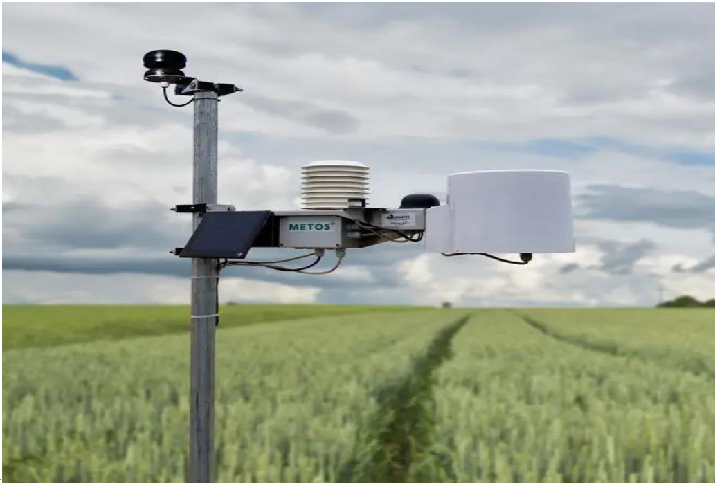
Photo 2. iMETOS 3.3 weather station
